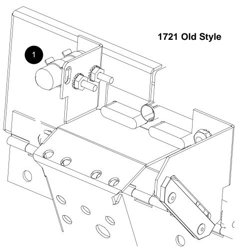
1. Remove existing tilt switch and supporting horse-shoe brackets. Retain screws and mounting plate.
